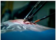
The instruments are real. The patient is not. It's artificial tissue — ideal for training. New robotic instruments, equipped with pressure sensors, will relay haptic information to surgeons at the console — helping them "feel," not just see, what they're operating on.
